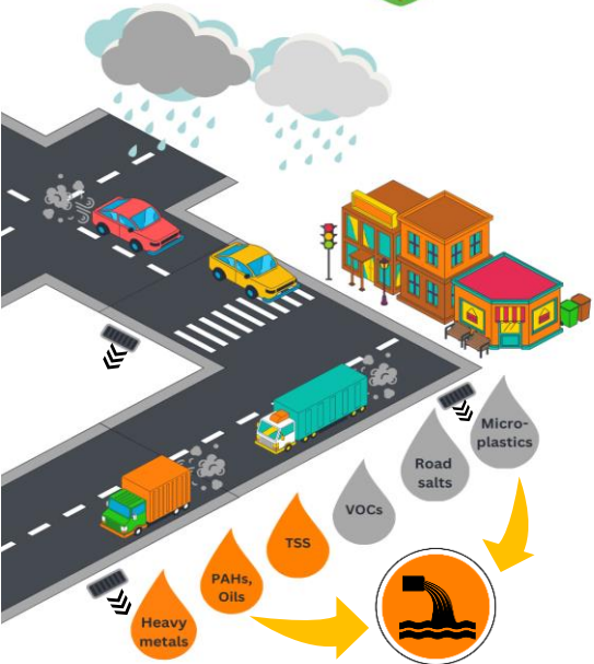
Fig 1. Contaminants from road surfaces get washed into drains and end up in waterbodies
