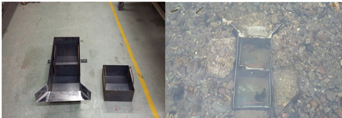
Figure 8: Sediment trap – in the laboratory and installed in the river
