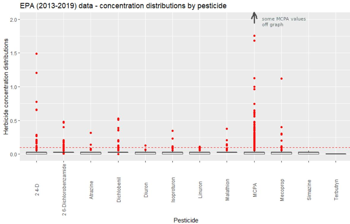
Figure 3: Box plots of EPA herbicide data concentration distributions ( $\mu\text{g/L}$ ) of key pesticides. Note: red dots show high concentration outliers and values below Limit of Reporting are treated as concentrations half that limit.
