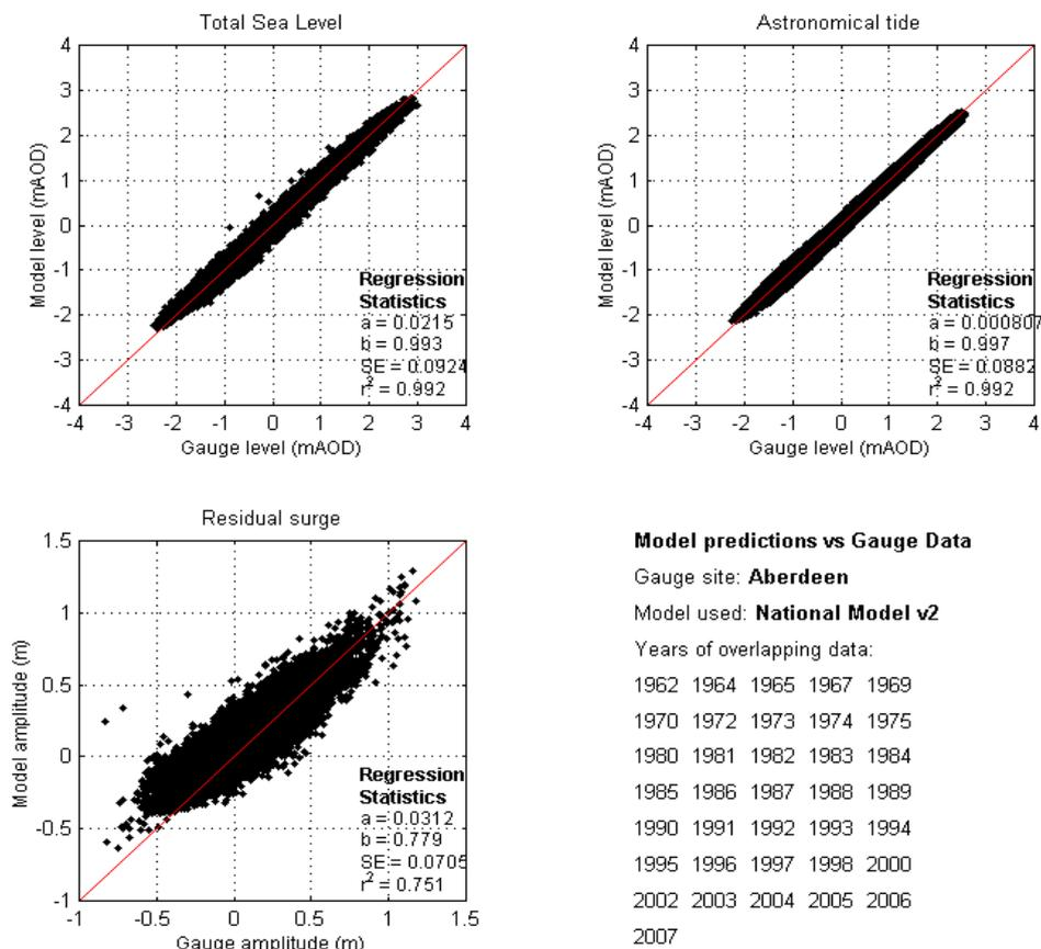
**Figure 4: Model vs Gauge comparison at Aberdeen**
