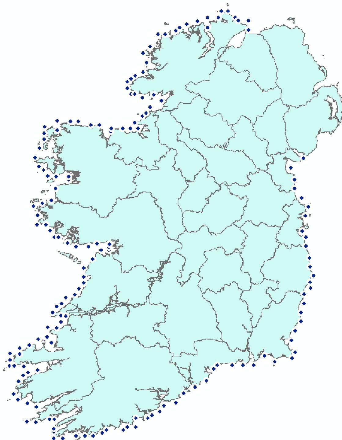
**Figure 6: Extreme sea level probability calculation sites for the JBA Irish ESL database**
