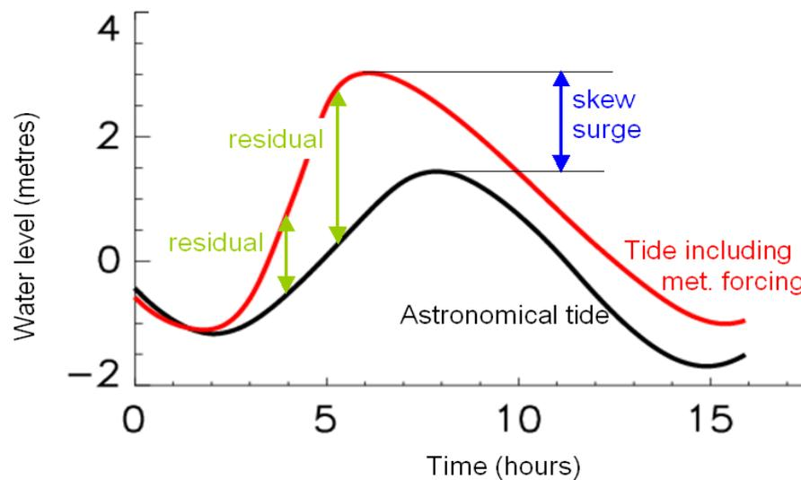
**Figure 3: Illustration of the Skew Surge parameter**
