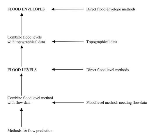
Figure 1 Methods for producing flood envelopes
